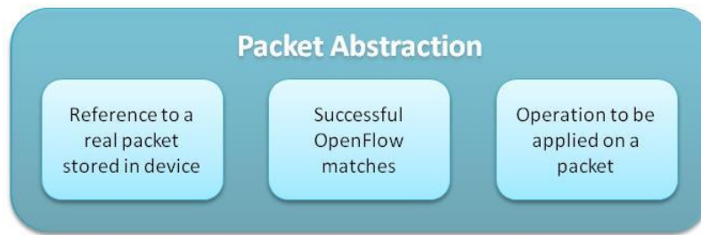
Figure 3.4 Cross-Hardware Platform packet abstraction object attributes
